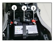
Check, using a voltmeter, that battery voltage is not less than 12.5 V.
